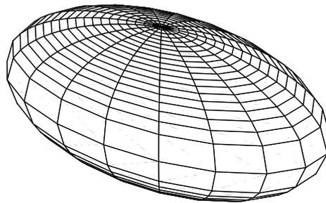
Abbildung 10: Ellipsoid  $\frac{x^2}{\alpha^2} + \frac{y^2}{\beta^2} + \frac{z^2}{\gamma^2} = 1$
